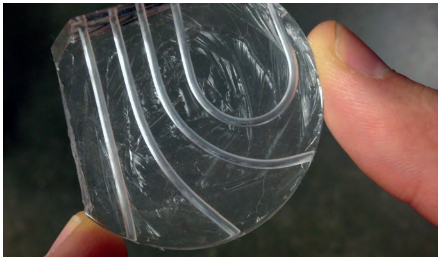
Figure 1. The simple fluidic transport system designed to help automate and streamline biopsy tissue sample preparation and handling. (Photo courtesy of the University of Washington).
