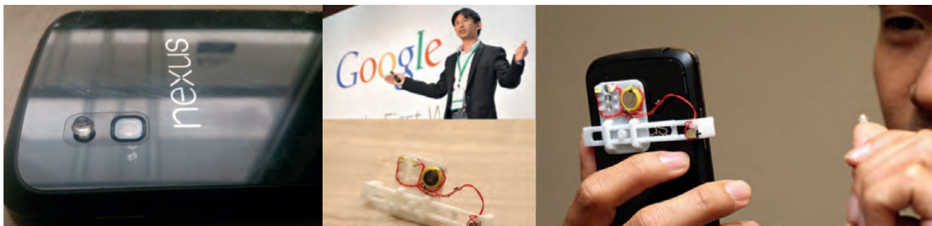
Figure 1. The mobile microscopy lens and lighting unit. Left, the lens in place on a smartphone camera. Middle, the lighting unit on its own and, right, attached to a smartphone.
