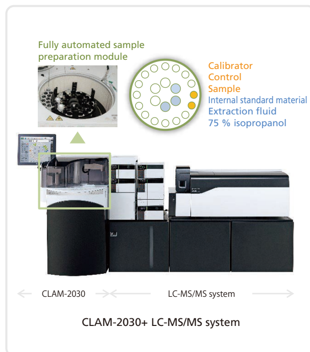
Fig. 6 Sample preparation for voriconazole using CLAM-2030
