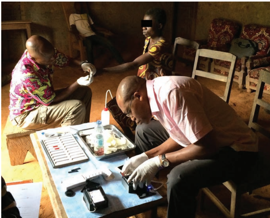
A pilot test in Cameroon of CellScope Loa, a mobile phone-based video microscope, found that the device was as good as conventional blood smears in detecting levels of the Loa loa parasitic worm. (Credit: Tom Nutman, NIAID).
